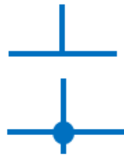
Wires not crossing
