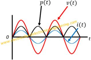
For a purely resistive load, the voltage and current are in series, and thus, the power at any instant is always positive. In electrical terms this positive power throughout the cycle indicates that power is continuously supplied to load.
