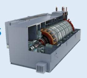
A synchronous generator is a synchronous machine used for converting mechanical power to ac electrical power. Synchronous generator is also known as alternator.
